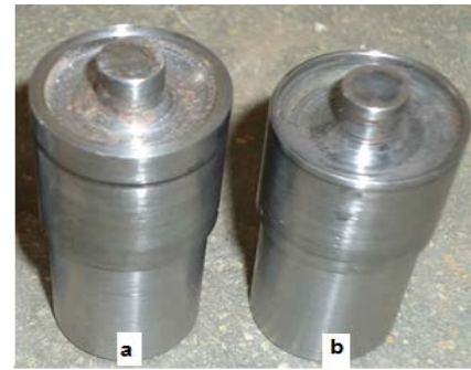
Fig.2. Tools with varying concave shoulder radius (a) R3, (b) R3.5
