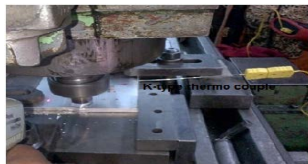
Fig.4. Set up showing the k-type thermocouple inserted into the base plate.
